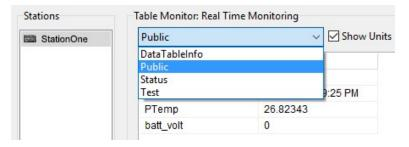
*PC400* users, click **Connect** <sup>SA</sup>, then **Monitor Data**. When this tab is first opened for a data logger, values from the **Public** table are displayed. To view data from other tables, click **Add I**, select a table or field from the list, then drag it into a cell on the **Monitor Data** tab.
